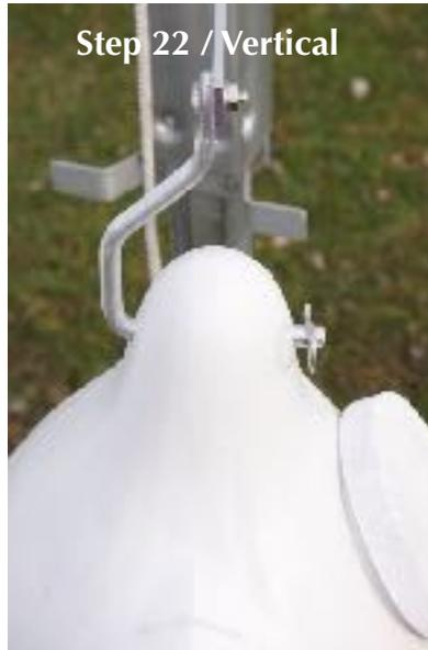
As seen in step 22 Horizontal. The pin of the GMA faces you. Be sure all the GMA's are level and tighten the from the bolt head.
