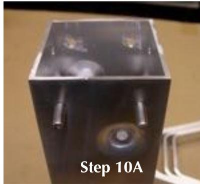
the arm so that the holes in the center of the gourd-hanging arm holes slips over the bolts on the hub. Thread the nuts on (10B)
