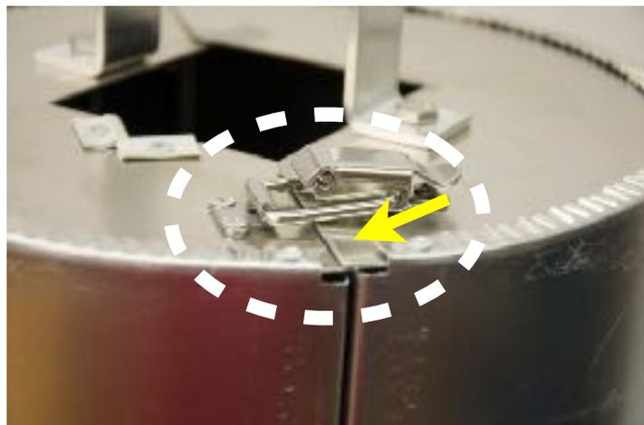
This EZ OFF is made to close shut in only one way, with the "latch" side to the top.
