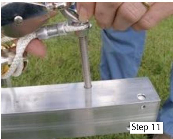
Thread the lock nut back on and tighten the nut all the way to the pole. Make sure that you orient the eyebolt so that open end is facing up, and that the eyebolt is
